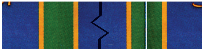
Fig 1.1 The left hand side is two impressions that are side by side on a printing plate. The right is where the plates meet when wrapped around the cylinder showing the cylinder gap.
